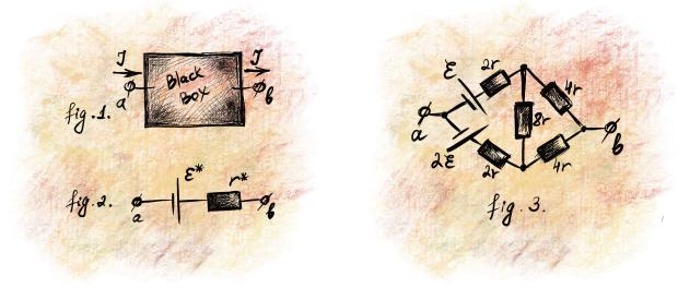
BB can be replaced by an equivalent EMF source (see Fig. 2).
