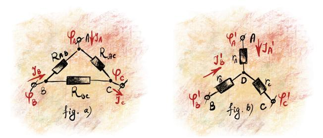
1.2 (0 points) Express the currents  $I'_A$  and  $I'_B$  in terms of  $r_A$ ,  $r_B$ ,  $r_C$ ,  $\varphi'_A$ ,  $\varphi'_B$  and  $\varphi'_C$ .
