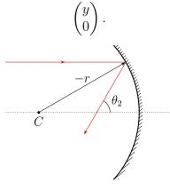
After reflection, it passes through the focus of the spherical mirror located at a distance r/2 from its vertex. Immediately after reflection, the beam height does not change, and the slope angle of the beam is
