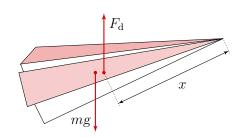
Lift force, gravity force, and drag force (can be neglected) act on an airplane when it flies horizontally. Let the point of application of the lift force be at a distance x from the nose of the plane.
