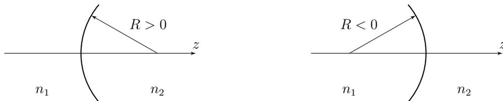
Let us consider the refraction of light on a spherical surface and find the matrix of refraction  $P$ . Let the ray pass from a medium with a refractive index  $n_1$  to a medium with a refractive index  $n_2$  (see fig.).
